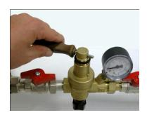
All the PE111.R filling units are tested before being packaged; during the proof they are pre-set at the outlet pressure of 1.5 bars; the outlet pressure can be easily modified when the valve is installed on the plant.
